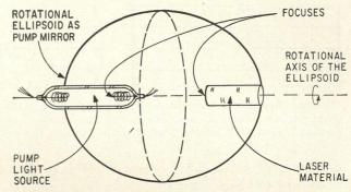
Light source is placed between focus and apex of the rotationally symmetric ellipsoidal pumping mirror. Reflection properties of ellipsoid cause light rays from the pump light source to be reflected through the focus-apex area at the opposite side of the ellipsoid where the laser material is located.
