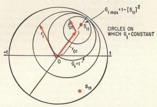
A graphical plot helps in design of an amplifier stage. Here the measured parameters  $s_n$  and  $s_n^*$  are plotted on a Smith chart. The upper point is  $s_n^*$ .
