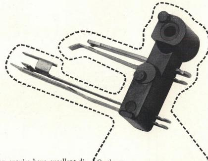
This phone dial relay switch used to be molded of soft-flow phenolic. Now it's made of a stronger, more versatile Plaskon® epoxy molding compound. Because of that, Western Electric was able to eliminate an expensive metal flange with no loss of strength. And at a substantial saving, considering the millions of parts that were made.
