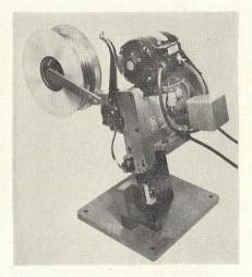
A solderless connector attaching machine has been developed for splicing leads. It utilizes a continuous spool of wire and completely eliminates the need for preformed connector strip. Connectors made from flat wire cost 80 cents per thousand as opposed to \$2.50 per thousand when made from preformed connector strip. This machine can operate with copper, brass, tinned brass, silver and aluminum wire.
