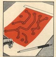
Cut a piece of the desired film large enough to cover area to be masked. Tape it down firmly at the top with dull-side up.
