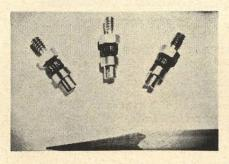
A significant reduction in size and weight of rectifiers with a 12-amp rating is possible with this miniature stud-mount series. Only 0.187 in. in diameter and 0.46 in. long, the unit weighs less than 1.5 grams. A 4-40 stud 0.19 in. long permits mounting to a heat sink. All units feature controlled avalanche characteristics and piv ratings up to 600 v are available.
