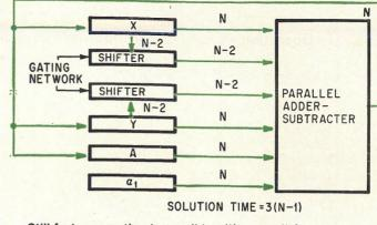
Still faster operation is possible with a parallel arithmetic unit that retains the simple serial shift-registers of the basic organization.
