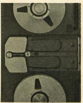
Advanced transport system features balanced tension direct drive. It eliminates belts, pulleys, gears, and pinchrollers and only the tape heads make contact with the oxide side of the tape.
