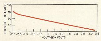
Threshold voltage can also be varied by applying a voltage at pin I.
