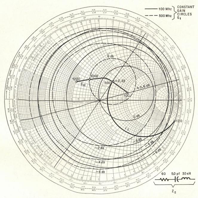
the input r<sub>1</sub> plane on the Smith chart. The impedance values at various frequencies between 100 and 500 Mhz are tried until an impedance that corresponds to an approximate constant—gain circle necessary for constant power gain across the band is found.
