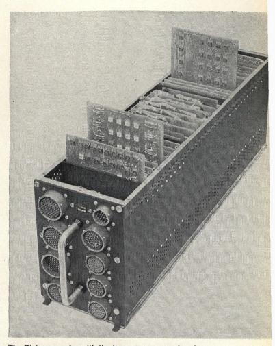
The Divic computer with the top cover removed and some of the circuit cards partly pulled out. The group of cards in the center carry the core-rope memory; portions of the rope are just visible. The ferrite core memory is on the module at the rear; only a few test points are visible.
