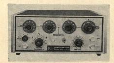
Series 4000 RC oscillators feature transient-free tuning, exact resetting by means of rotary switches, harmonic distortion less than 0.01%, frequency response within  $\pm 0.01$  db, amplitude stability of  $\pm 0.01\%$  per hour, and voltage calibration accuracy of  $\pm 0.25\%$  without a meter. The solid state units cover frequencies from 0.001 hz to 100 khz.
