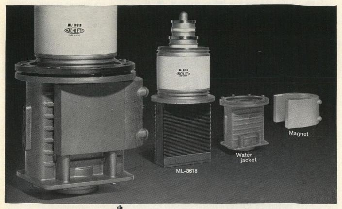
ML-8618, Machlett's new magnetically beamed water-cooled triode, provides high power gain, high plate efficiency and maximum cathode utilization. Electron trajectory from cathode to plate is magnetically controlled to greatly reduce electron interception by the grid . . . and therefore decrease grid current and heating and allow significantly higher performance levels.
