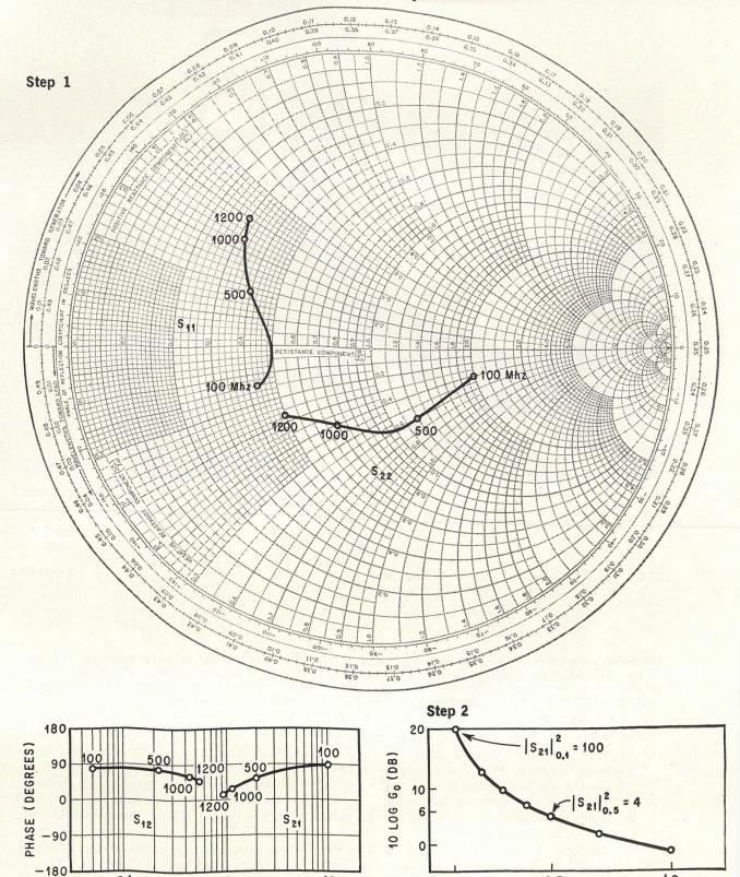
From the measured data transducer power gain is plotted as decibels versus frequency. From the plot an amplifier of constant gain is designed. Smith chart is used to plot the scattering parameters.
