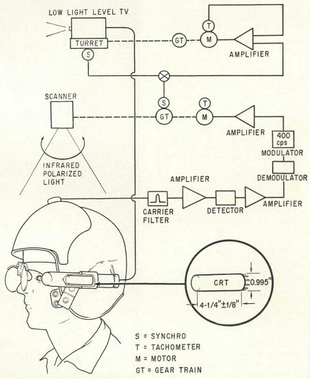
Optoelectronic servosystem allows pilot to control television camera in nose of helicopter by movements of his head. Transmitter in scanner emits light in the near-infrared region that is polarized and is scanned to determine its phase and amplitude. The monitored signal is used to drive a servosystem that controls the camera's position.
