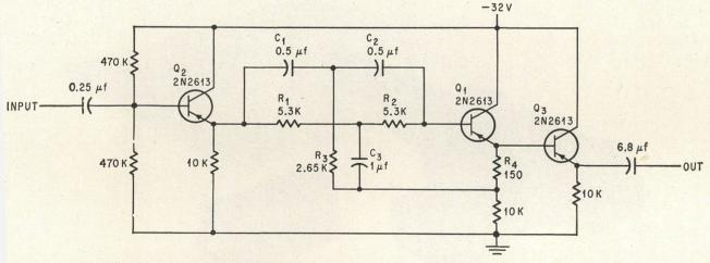
Transistor  $Q_2$  provides feedback for the parallel T-notch filter. Values shown for components are designed for 60 hertz. For 120 and 180 hertz decrease capacitor  $C_1$ ,  $C_2$  and  $C_3$  values proportionally. Control of the rejection bandwidth is provided if the 150-ohm resistor is made variable to 680 ohms. This is done with a potentiometer.
