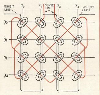
winding therefore selects a single core in each plane; if the planes are horizontal, the selected cores will be in a vertical column through the stack. Each plane corresponds to one bit in a word, and contains one bit of every word in the memory. Each plane has its own individual sense winding and inhibit winding passing through every core in the plane.
