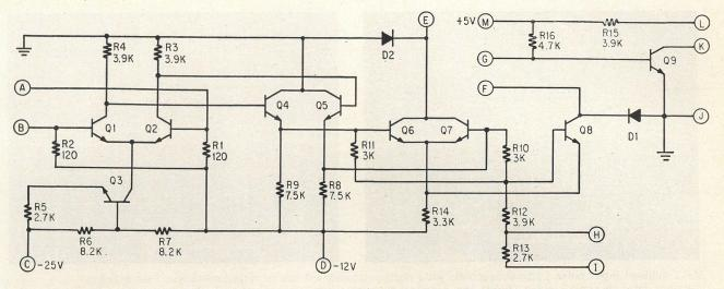
Adjustable threshold and choice of positive or negative output pulse are features of this general-purpose sense amplifier. The threshold is established by the connection of pin H or I to ground or to a positive or negative voltage, directly or through a resistance; thus there are three ways to adjust it. For a negative output pulse, pins F and G are connected together; for a positive output pulse, pins E and G are connected.
