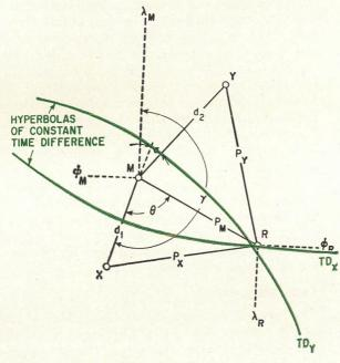
Two spherical triangles must be solved and the results transformed into position and course data in a hyperbolic coordinate system. The symbols  $\phi$  and  $\lambda$  represent latitude and longitude, respectively; the subscripts represent the master station, M, and the receiver, R.
