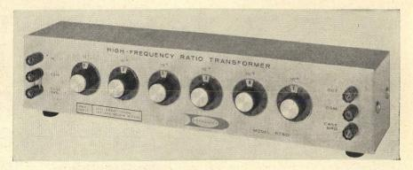
The first commercially available ratio transformer capable of operating to 500 kilohertz is claimed by the Dytronics Co. The model RT-501 inductive voltage divider can resolve an a-c input voltage into more than one million parts. The accuracy of the divider's transformation ratio is within 0.0005% near the lower operating frequency limit of 4 khz and 0.09% at the upper frequency limit of 500 khz.
