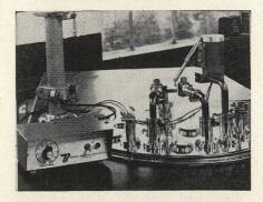
An accessory for thin-film evaporators permits continuous, controlled feeding of coating material to a hot source or an electron beam gun. Known as a vibratory feeder, the accessory makes it possible to obtain uniform, homogeneous film formation even with varying vapor pressures of coating material compositions and alloys.
