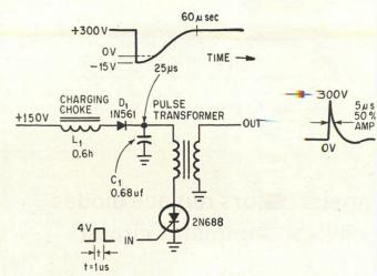
Capacitor  $C_1$  is charged by the supply three ugh chargin choke  $L_1$  and diode  $D_1$  to 300 volts. An incoming trigger pulse turns on the scr, discharging  $C_1$  three ugh the princ of the pulse transformer and producing a 300-volt spil output pulse. The ringing of  $L_1$  and  $C_1$  turns off the scr.
