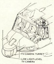
Bell envisions several uses for its tv system: pilots can fly by it, direct armament and use it for surveillance.
