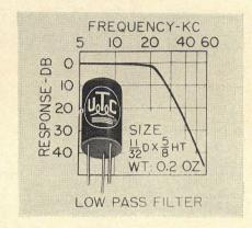
Ultraminiature low-pass filters have the same physical configuration as the DO-T family of audio and power transformers, having a diameter of only  $\frac{1}{32}$  in., height of  $\frac{5}{8}$  in., and weight less than 0.2 oz. Its size makes it ideal for printed-circuit applications. The metal-encased, hermetically sealed filter is designed, manufactured and tested to complete MIL-T-18327B specification.
