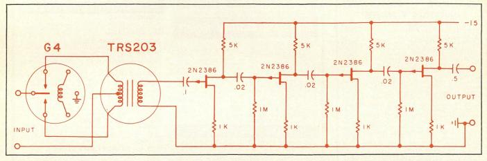
The FET amplifier has remarkable low noise performance. Tubes — and transistor junctions — have at least one thing in common — the noise power increases as the frequency goes down. This means a lot of litter near DC, making readings at less than 100 nanovolts about impossible, unless the amplifier bandwidth is severely restricted. You can read 10 nanovolts with this circuit with wide band response.
