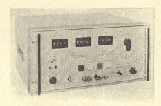
Limit bridge model 5350 provides simultaneous limit decisions for both series capacitance and dissipation factor at 120-hz or 1,000-hz test frequencies, and completely eliminates stray capacitance effects due to bias supplies, capacitance to ground, shielded leads, and other causes. A zero to 300-v bias supply can be used with no effect on either capacitance or dissipation factor measurements. The company claims this is the first bridge to allow this type of measurement.
