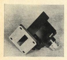
Added packaging flexibility is provided with the incorporation of integral waveguide adaptors on the company's standard coaxial ferrite circulators and isolators. A typical example is the ICC-199 isolator which covers 5.9 to 6.3 Ghz and has a waveguide input and a type N female coaxial output.
