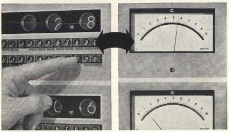
Once the Bridge is trimmed, a series of front-panel range push-buttons are suppressed in sequence until a reading is obtained on the meter. Setting up the first one or two digits of this reading on push-button decade controls gives the
