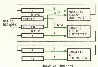
The fastest and most complex layout uses both parallel arithmetic units and parallel processing from all registers. This organization also costs the most.
