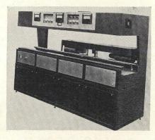
Series 4000 dual wave soldering machine has been developed for the high production and efficient soldering of circuit assemblies.
