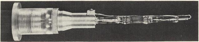
Ruby laser with repetition rate of 100 hz uses ellipsodial pumping mirror, 1-inch-long ruby rod, high-pressure mercury-vapor flashtube. Absolute output efficiency is 0.22 %. Flashtube, in photograph has preadjusted, interchangeable holder and electrical plug-in. It can be produced cheaper than xenon units.
