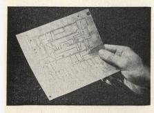
Materials developed for multilayer p-c boards permit maximum design flexibility and consistent, high-quality production. The product package consists of a thin copperclad epoxy-glass laminate, designated Textolite Grade 11685, designed for use with three new epoxy-resin impregnated glass cloth bonding sheets — Grades
