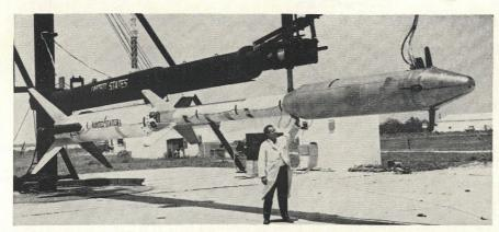
Project Scanner payload designed to gather information on the earth's horizon to orient future satellites more precisely.
