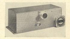
Low noise and high stability characterize this X-band solid state source. The output can be remotely switched between three discrete frequencies all above 10 Ghz in a 150-Mhz bandwidth.
