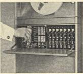
Front-access universal housings assure unmatched flexibility; accept plug-in circuit cards for Digital, FM, or Direct electronics.
