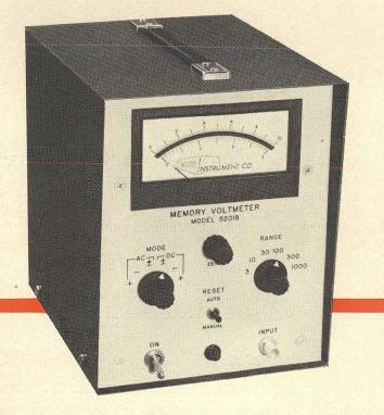
The Model 5201 memory voltmeter is a dc to 20 mc instrument which measures and stores indefinitely the maximum peak voltage applied, including continuous or one shot pulses as short as 50 nanoseconds. A memory reset-switch on the front panel allows the 5201 to monitor peak values of a varying waveform, either positive or negative going.
