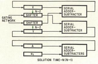
A somewhat faster and more complex organization is parallel processing. It increases the speed and requires additional hardware; serial arithmetic is retained. The arrows in color refer to a number of parallel lines.
