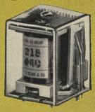
Type LB Relay has tinned nickel silver terminals for direct PCB mounting. Volume: 1.33 cubic inches. Maximum mounted height, 1.24 inches. Relay shown actual size.
