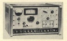
A broadband sweep generator, model 900-C, is designed for sweep frequency analysis of the response of various electronic circuits. The instrument permits observation of the entire frequency response of the unit under test (up to a 400-Mhz bandwidth), or will examine a narrow 10-khz segment. It can be used to make qualitative analysis of the response of a wide range of electronic devices such as receivers, amplifiers, filters, transformers or transmission lines.
