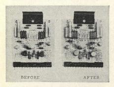
A conformal coating has been added to the company's line of quality resin products. TC-3050 coating was developed to give p-c boards the best environmental protection possible, while giving the applicator a broad selection of application methods and curing schedules.
