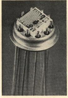
The Hughes Aircraft Co.'s Microelectronics division has developed a d-c amplifier with an output voltage range of ±36 volts. The company claims the hybrid integrated circuit amplifier, designated HMC 1148, outperforms any unit its size. Hughes says amplifiers with monolithic circuits usually can deliver only about ±15 volts.
