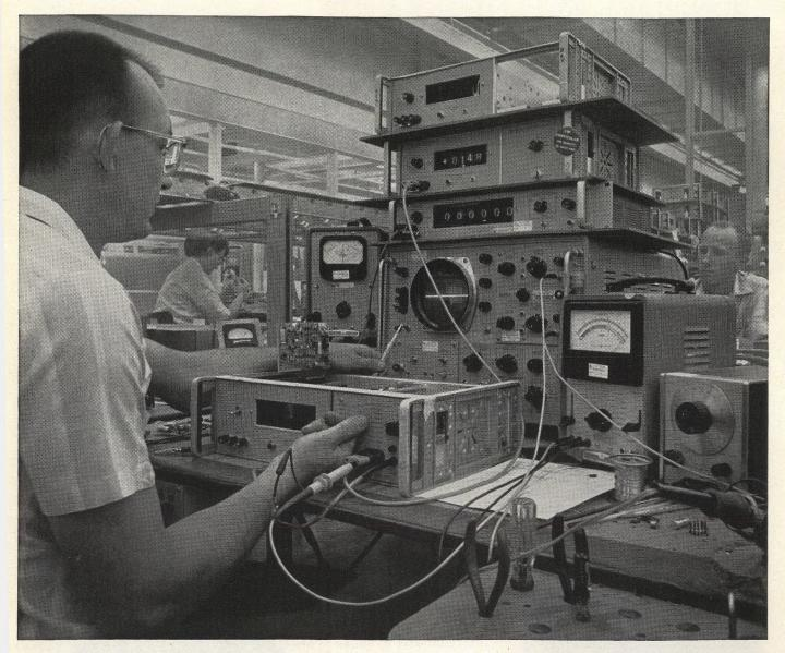
That's "testing" backwards. And that's what we do to every Hewlett-Packard 3439A and 3440A. Test it forwards, backwards, inside and out. ■ Here you see it going through complete testing and calibration after assembly. Every circuit board is checked, and then the entire instrument is calibrated to be sure it meets specifications. ■ But that's just the beginning. From here it goes into a 50°C
