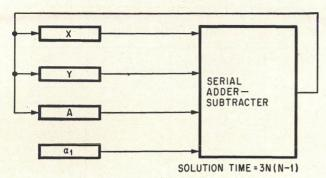
The simplest organization for a Divic computer is when data is processed serially, and arithmetic operations are performed serially.
