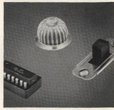
RESISTS SHOCK... TI molded integrated circuits resist impacts that would smash metal packages and shatter ceramic packages as shown in top photo. You benefit from fewer failures in handling accidents and greater reliability in service. The solid molded construction gives extreme resistance to acceleration, vibration and shock as proven in acual test (see opposite page).
