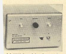
odel 1202-3 wideband amplifier, ich is composed of silicon planar vices, uses feedback to achieve it response and gain stability. in is adjustable from 10 to 100. Equency response is 5 hz to 10 1z at 20-db gain and 10 hz to 1
