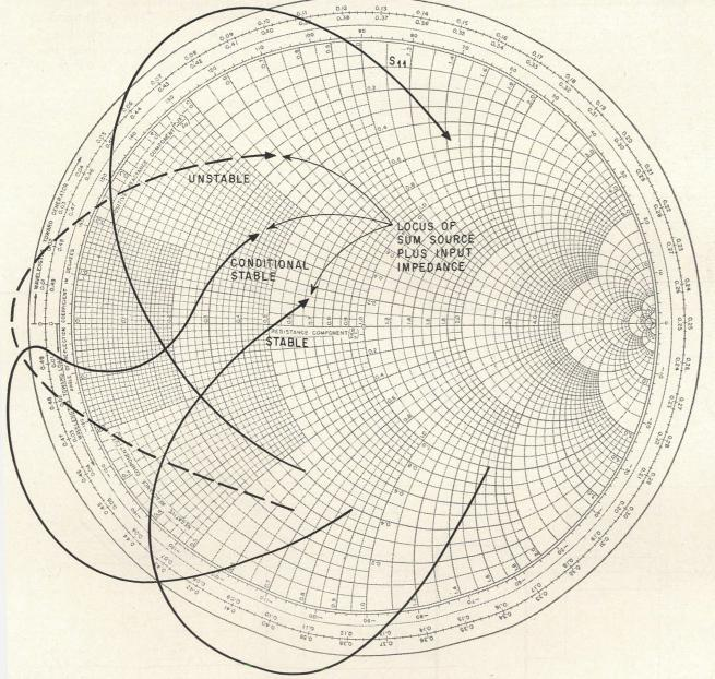
Amplifier stability is determined from scattering parameters and synthesized source and load impedances.
