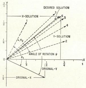
Typical rotation operation is shown plus the steps toward its solution with the Volder algorithm. The angle after the rotation is approached with steadily decreasing steps; the magnitude steadily increases with each step and in general will require correction, the amount of which depends on the computer word length and the number of steps
