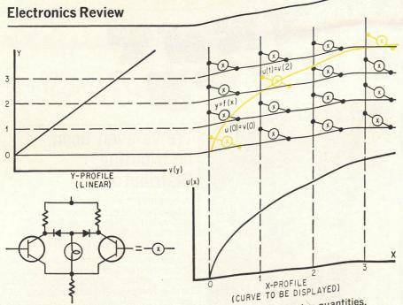
Paramosaic, a prototype of a digitally controlled display for analog quantities.
