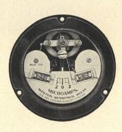
Model 723 Sensitrol—sealed; shielded; internal reset; solder terminals; single or double magnetic contact; ranges as low as 1-0-1 μa.
