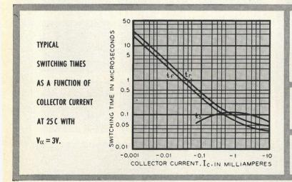
Fastest switching transistor available in the 1 to 100  $\mu$ A range.
