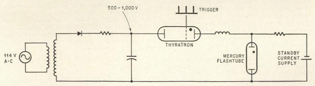
Trigger pulses on the thyratron determine the pumping frequency (50 to 120 hz) of the flashtube in this simplified schematic of the commercially available Siemens power supply.
