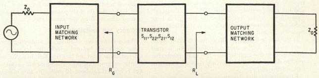
To design an amplifier stage, source and load impedances are found to give the gain desired. Then impedances are synthesized, usually as matching networks between a fixed impedance source or the load and the device. When using s parameters to design a transistor amplifier, it is advantageous to distinguish between a simplified or unilateral design for times when  $s_{12}$  can be neglected and when it must be used.
