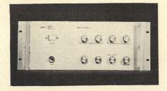
A video plotter has been developed to display graphic information directly on the screens of standard television monitors, with resultant increased flexibility as compared with conventional paper recorders. The traces produced by the model 401 are bright and nonfading, but can be completely erased in a fraction of a second. Signals from the 401 can be intermixed with those from tv cameras, flying spot scanners or other video sources to produce highly complex displays.
